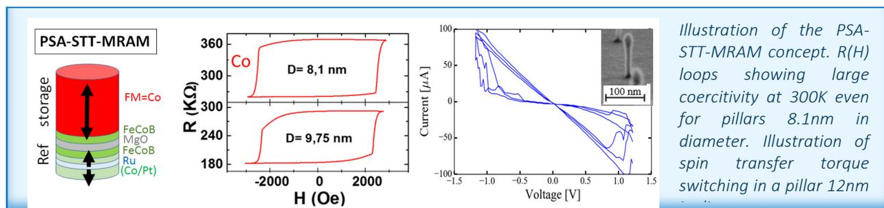
*Illustration of the PSA-STT-MRAM concept.  $R(H)$  loops showing large coercivity at 300K even for pillars 8.1nm in diameter. Illustration of spin transfer torque switching in a pillar 12nm*
