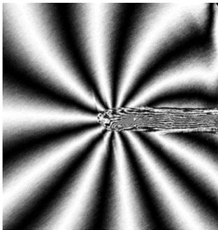
Iso-lines of magnetic phase arising from a Ni nanowire in a magnetic state close to saturation. The dense lines within the nanowire are indicative of magnetization, while the lines in vacuum pertain to the stray field of dipolar origin created by the wire.
