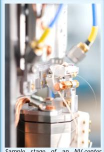
Sample stage of an NV-center microscope designed at SPINTEC
