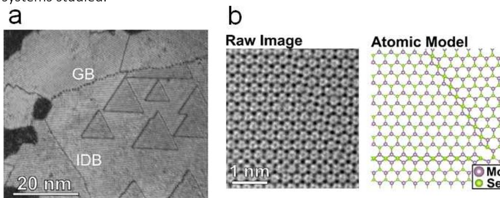
Figure 1: Aberration-corrected transmission electron microscopy (AC-TEM) image of a MoSe<sub>2</sub> layer; (a) overview of grain and inversion domain boundaries and b) atomic structural analysis of inversion domain boundary [2].
