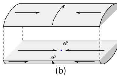
Open sketch of a domain wall in a cylindrical nanowire, embedding a Bloch-point at its core
