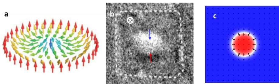
Figure 1: a) Schematic representation of a magnetic skyrmion [1]. b) XMCD-PEEM image of magnetic skyrmion (130 nm diameter) at room temperature and zero magnetic field in an ultrathin Pt/Co/MgO nanostructures [3]. c) Spin structure from micromagnetic simulations.
