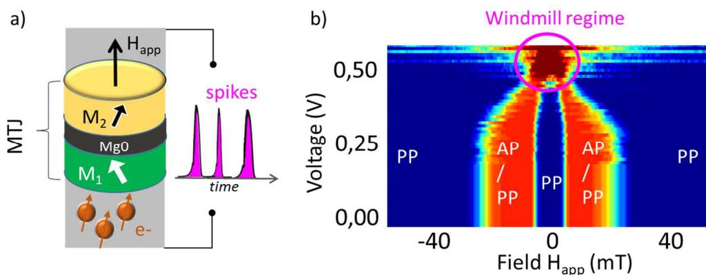
Figure 1: a) Schematics of two free magnetic layers weakly coupled, their interaction can be controlled by the mutual spin torque effect. b) Experimental voltage-field state diagram of perpendicular magnetic tunnel junction pillar having 100nm diameter, showing the windmill regime.
