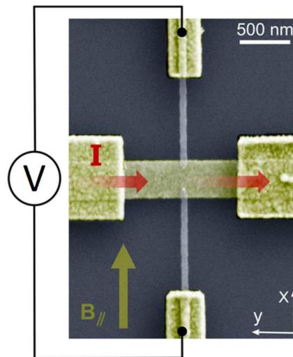
Figure 1 : Example of a nanodevice made in our team allowing the electrical measurement of the charge current - spin current conversion [4]. The charge current travels along the horizontal track in the spin-orbit material, generating a spin accumulation, and the vertical ferromagnetic electrodes probe this accumulation.
