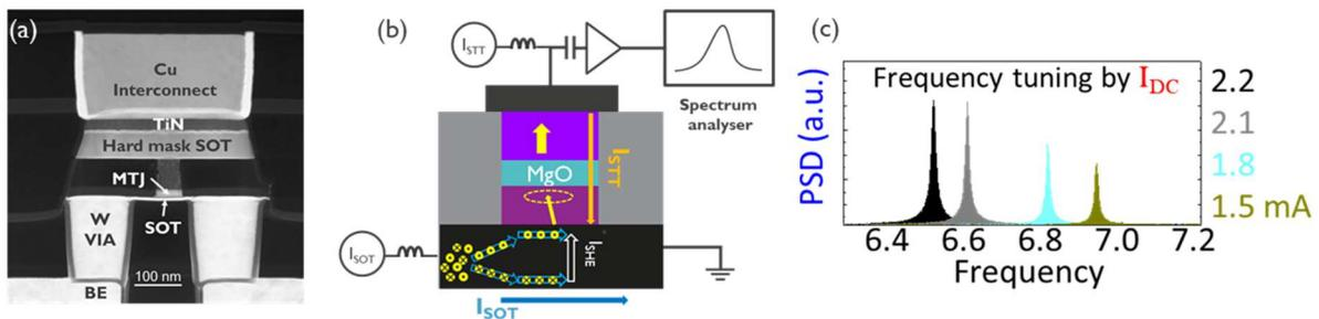
Figure 1 : (a) TEM Cross section of an SOT-MTJ that will be used in this project [6], (b) electrical scheme of a SOT/STT-STNO, (c) power spectrum of magnetization oscillation induced by STT.
