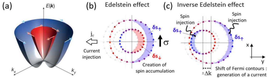
Figure 1: a) Band structure of a Rashba system, with two Fermi contours having opposite spin helicities. Charge-spin (b) and spin-charge (c) conversion: in (b) the injection of a charge current  $J_c$  along  $y$  shifts the Fermi contours and generate a spin density  $\sigma = \delta s_{\uparrow} - \delta s_{\downarrow}$  along  $x$ . In (c) the injection of a spin density  $\sigma$  along  $x$  shifts the contours along  $y$ , creating a finite charge current.
