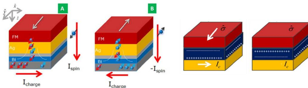
Figure 1: Spintronics devices associating two types of components : ISHE/Rashba metallic pillars converting vertical spin current into horizontal charge current (left) and Magnetoelectric insulating capacitors allowing to switch the magnetization of nanomagnets (right)
