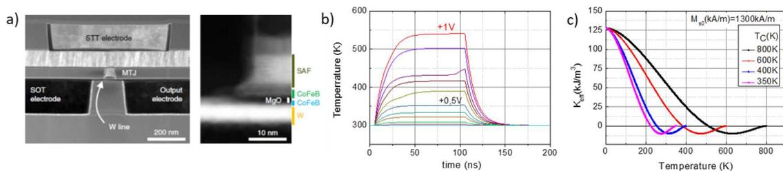
Figure 1: a) TEM Cross section of a SOT-MTJ [3]. b) Typical time evolution of the temperature of the MTJ sample for different bias voltage pulses. c) Temperature-induced variation of the effective anisotropy of a CoFeB free layer depending on its Curie temperature  $T_c$ .
