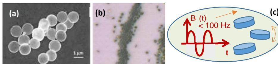
Figure 1: Magnetic particles imaging. (a) SEM image of magnetic particles ( $\varnothing$  1.3  $\mu\text{m}$ , 60 nm-thick) from PTA, Spintec [2] (b) Optical image of self-polarization of particles in a fluid (acetone) in zero magnetic field [4] (c) Sketch of particles actuation by alternating magnetic field in an agarose gel.
