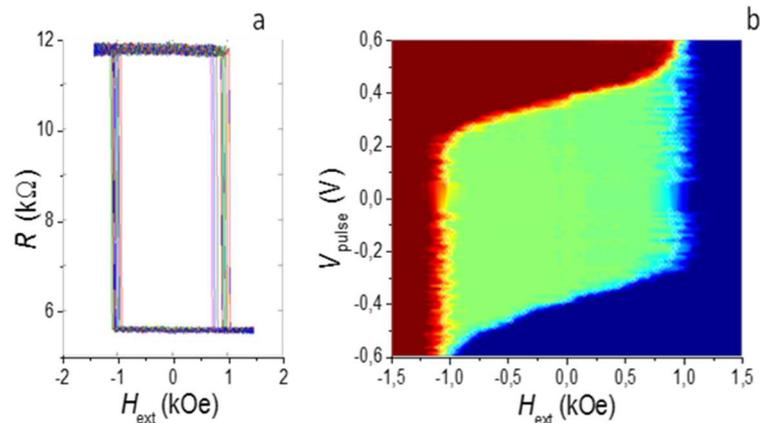
Figure 1: a) A Magneto-Resistive (MR) hysteresis cycle measured on a perpendicular anisotropy tunnel junction showing the variation of the resistance and two distinct resistance states [1]. b) A state-phase diagram plot of the same junction when applying current pulses. The color code shows the resistance state, blue for low and red for high resistance, with green being the bi-stable region for memory cell.
