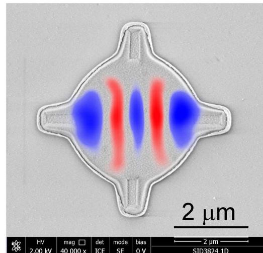
Figure 1: SEM image of a suspended drum-like YIG resonator with an overlay of a spin wave pattern measured on the same structure by TR-MOKE.
