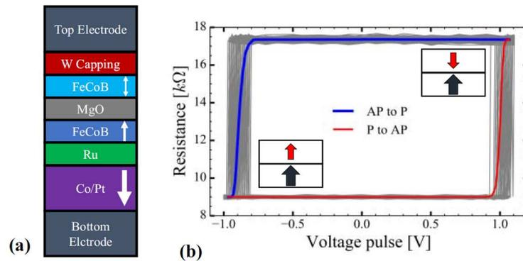
Figure 1: a) Typical magnetic stack of a perpendicular anisotropy magnetic tunnel junction used in non-volatile memory MRAM cells. b) Electrical characterization of 500 hysteresis loops showing individual voltage loops in grey and their mean value in blue-red [1]. The dispersion of the witching voltage allows for the extraction of thermal stability parameters.
